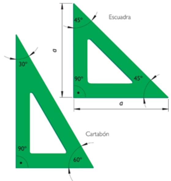
To draw parallel and perpendicular straight lines you simply slide the first triangle (escuadra) over the hypotenuse of the second triangle (cartabón).
