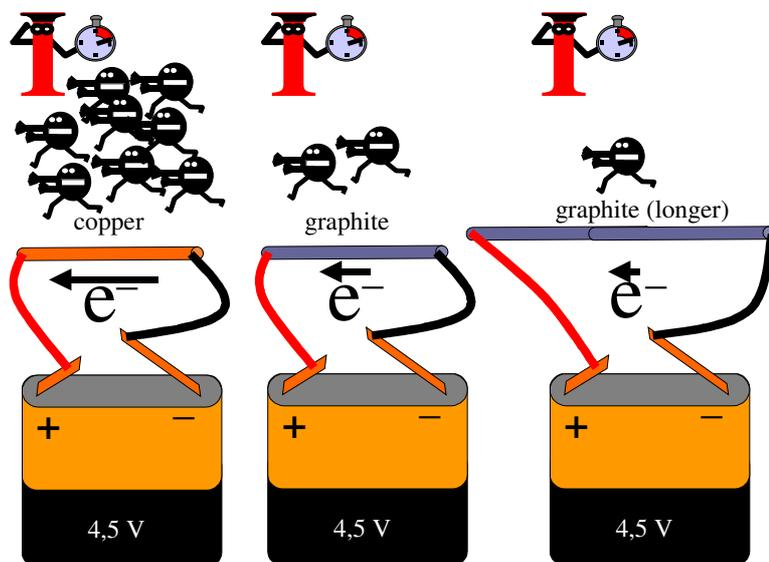
The opposition or obstacles that hinder the flow of electrons through a conductor is called resistance. It is represented by the letter **R** and is measured in **ohms ( $\Omega$ ; 1  $\Omega$  = 1 V / 1 A – see Ohm's law)**.
