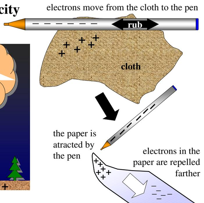
Alternative ways to separate electrons farther from positive charges are chemically (in batteries) or by electromagnetism (in alternators or dynamos). Consequence of this separation process is the creation of an **imbalance** between two 'points' or **poles**: the **negative pole**, the 'point' where electrons has been moved, and the **positive pole**, the 'point' where the positive charges remain.
